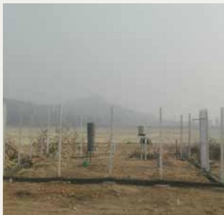
Tipping bucket rainfall gauge at Chisapani Bazaar (above). The Department of Hydrology and Meteorology is progressively replacing older rainfall gauges with automatic weather stations that send real-time weather information across the mobile networks.
